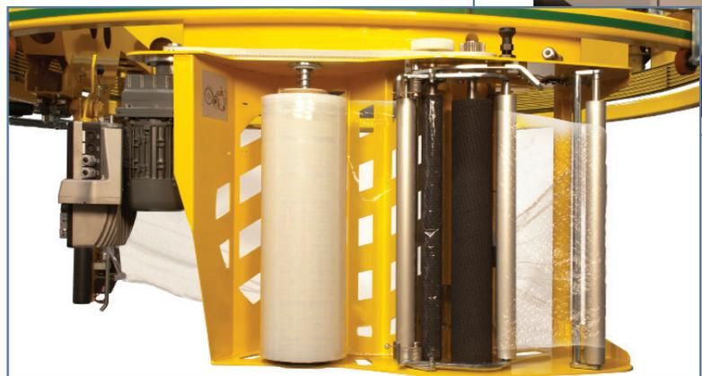
*The "S" style film carriage is easy to load and reduces downtime. It features a very efficient and consistent power pre-stretch system that helps minimize film usage.*
